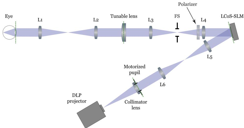
**Fig. 1.** Schematic of the AOV system. Lenses L1 to L6 – achromats with focal lengths of 100 mm. Planes conjugated to the entrance pupil of the system are shown with a green dotted line. Further explanation is given in text.
