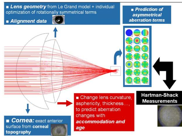
Fig. 2. (Color online) Schematic diagram of the procedure to build up the individualized eye models used in this work.
