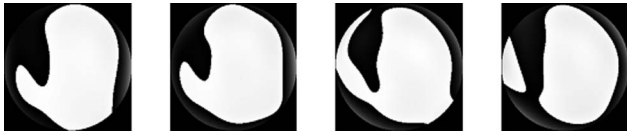
Fig. 7. “Residual” WAs for the high-power laser beam using the first HS image (time = 0) as a reference. Left to right panels correspond to the time sets of 1 s, 15 min, 1 h, and 3 h.
