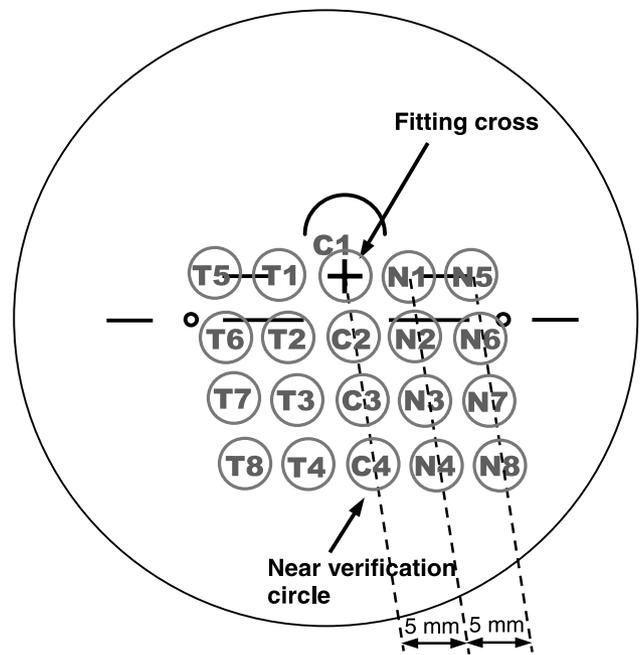
**Figure 2.** Measured zones in the PPLs with 4.0-mm in diameter.
