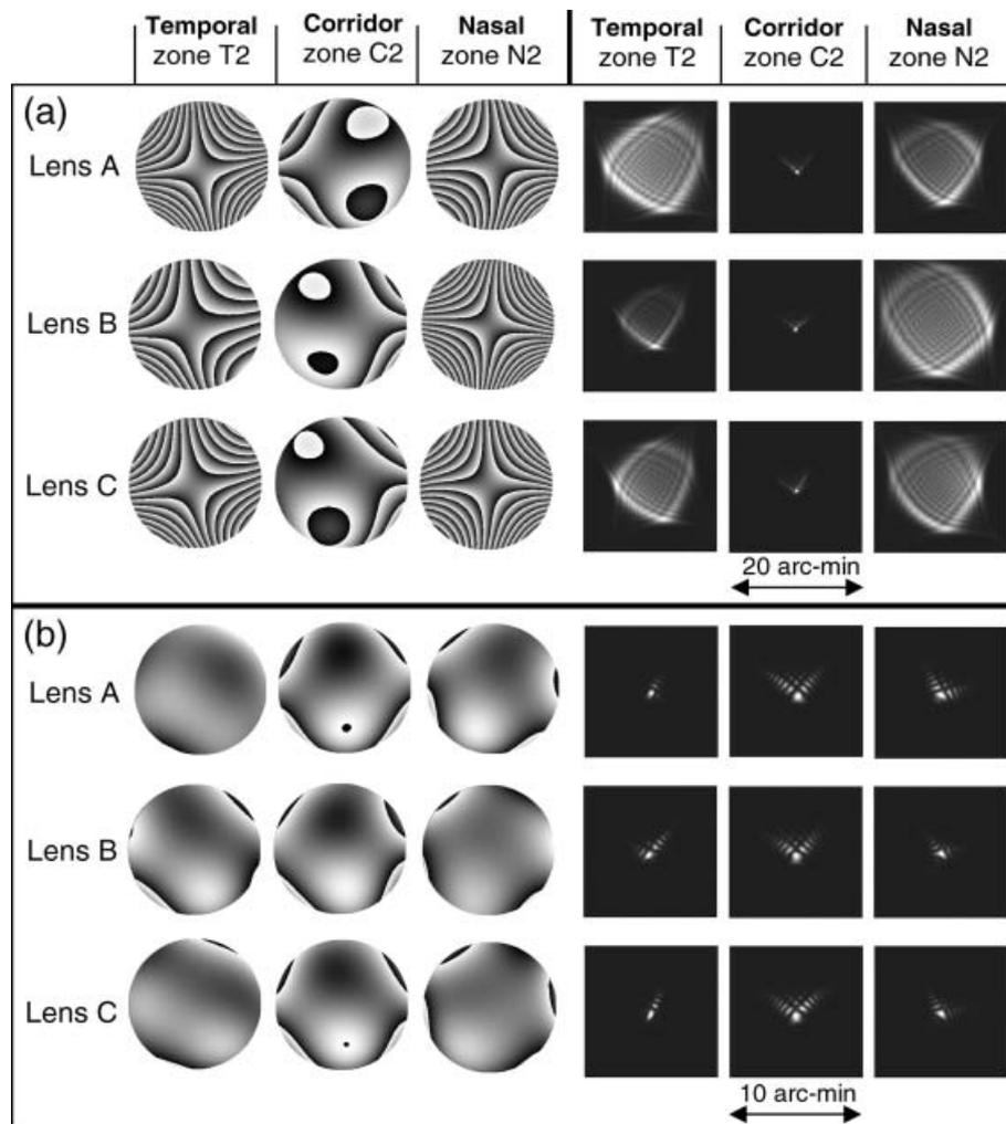
**Figure 3.** A modulus  $2\pi$  representation of the WA maps and the associated PSFs, at three intermediate zones ( $C_2$  at the corridor,  $N_2$  and  $T_2$  at the nasal and temporal side), as examples of the twenty tested zones, for each PPL. (a) Considering defocus zero. (b) Considering defocus and astigmatism zero. 6.0-mm pupil diameter.
