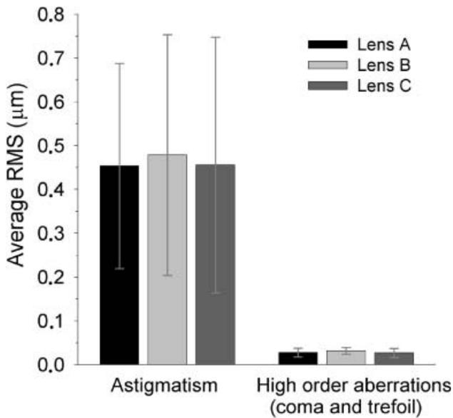
**Figure 7.** Average RMS of all tested zones of the lenses, for astigmatism and high order aberrations (coma and trefoil) with 4.0-mm pupil diameter. The error bars are the standard deviations. In the case of astigmatism, this parameter denotes how soft or hard the design is.
