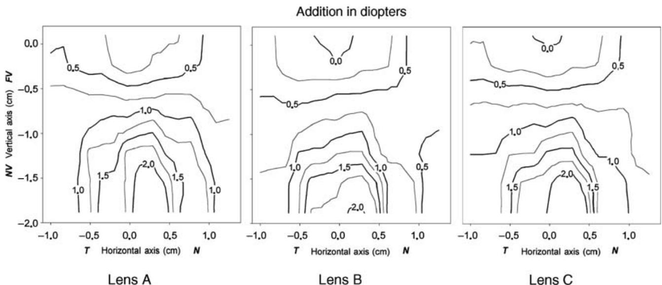
**Figure 8.** Contour plots of addition for 4.0-mm pupil diameter.
