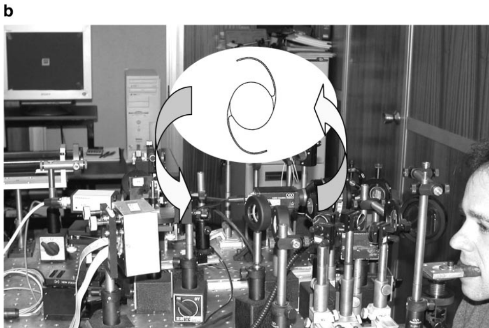
FIGURE 1. (a) Diagram of the AOVS. (b) The actual experimental system that reproduces the optical properties of a customized IOL.
