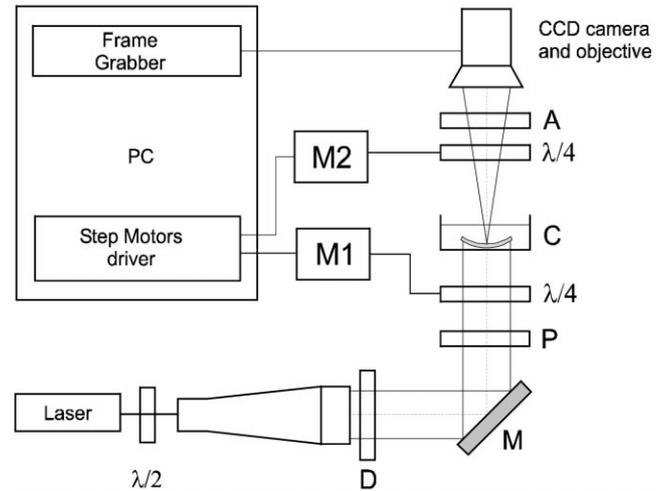
**Figure 1.** Schematic diagram of the Mueller-matrix imaging polarimeter used for *in vitro* measurements of corneal polarization properties.  $\lambda/2$ , half-wave plate; D, diffuser; P and A, horizontal linear polarizers;  $\lambda/4$ , quarter-wave plates; C, sample (*in vitro* cornea); M, mirror; M1 and M2, step motors.
